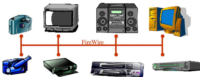
Figure 1: An Example of interconnected AV devices.
