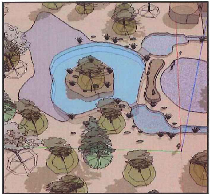
Concept sketch of constructed wetland with biofiltering plants, and avian island to promote biodiversity.
