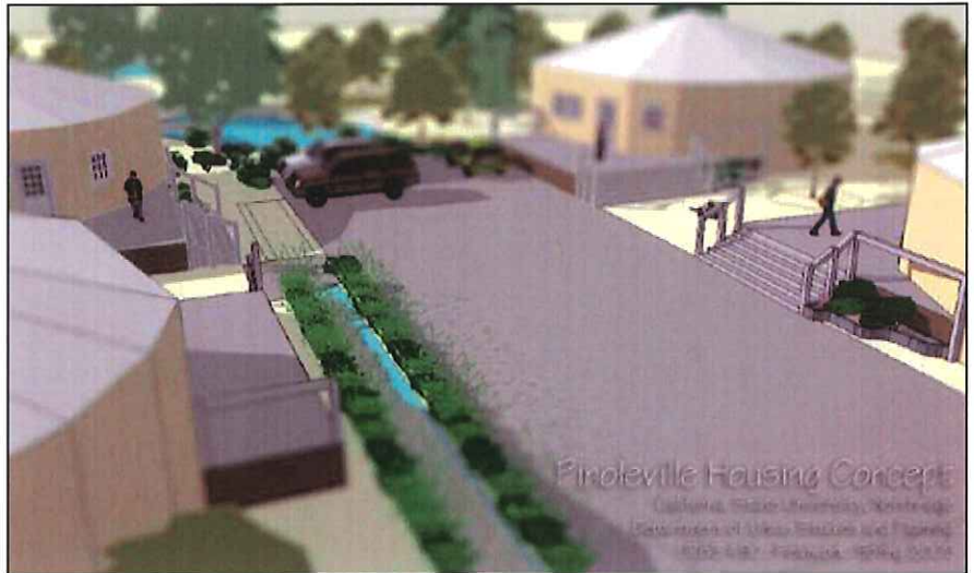
Potential cluster housing design rendering with yurt style housing, shared Parking and stormwater swales.
