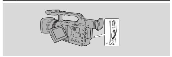
The zebra pattern is a series of diagonal stripes that appear in the viewfinder to highlight areas of overexposure. Use it as a guide to set the aperture (iris) and shutter speed.
