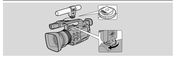
The high sensitive Directional Stereo Microphone DM-50 attaches to the "5" advanced accessory shoe for cable-free operation and is powered by the camcorder's power supply. Use it when recording or dubbing audio.
