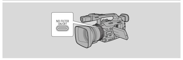
On bright days or when recording very bright scenes, despite the iris being at its smallest aperture, blurring of the image may occur. If this happens, using the ND filter should remove this problem.
