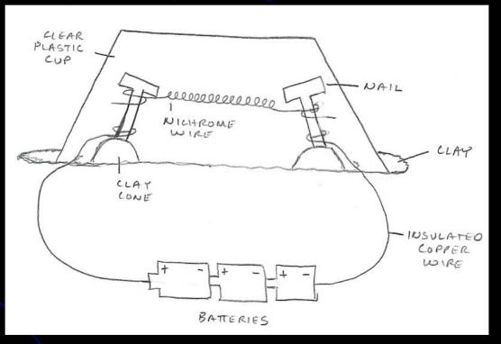
Connect one battery to the circuit and record your observations. Keep adding batteries until you see the Nichrome Wire give off light.
