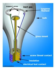
When the bulb is hooked up to a power supply, an **electric current** flows from one contact to the other, through the wires and the filament. Electric current in a solid conductor is the mass movement of **free electrons** (electrons that are not tightly bound to an atom) from a negatively charged area to a positively charged area.
