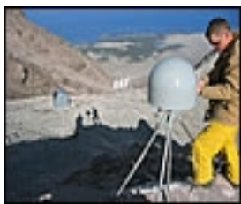
GPS receiver installation
