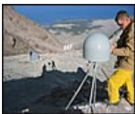
GPS receiver installation
