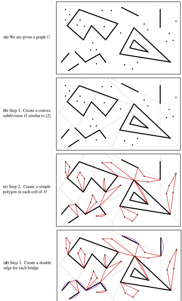
Steps 1–3 produce a 2-edge-connected *multigraph*. Step 4 transforms it into a 2-edge-connected *simple* PSLG by substituting or removing double edges (as in [1]).
