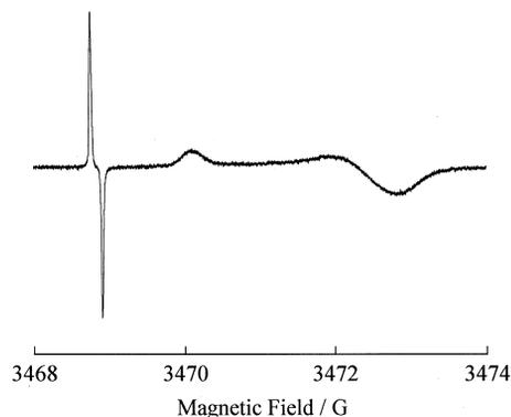
Fig. 2. In-phase ESR spectrum of irradiated vitreous silica, broad resonances near 3470 and 3472 G, and a single crystal of fluoranthenyl radical cation salt  $(FA_2)^+PF_6^-$ , narrow resonance near 3469 G. The modulation frequency is 210 kHz. The narrow lines display the two microwave sidebands and an absence of a central component.
