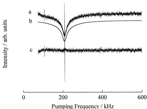
Fig. 3. (a) A typical in-phase TMFESR spectrum of  $\gamma$ -irradiated vitreous silica, with the field set at 3472.9 G. The observing frequency is 210 kHz and pumping frequency is swept from 61 to 586 kHz. (b) The best fit to the observed signal which is composed of the absorption of two Lorentzian lines. (c) The difference between the experimental spectrum and the best fit.
