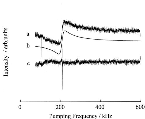
Fig. 4. (a) A typical out-of-phase TMFESR spectrum of  $\gamma$ -irradiated vitreous silica, with the field set at 3472.9 G. The observing frequency is 210 kHz and pumping frequency is swept from 61 to 586 kHz. (b) The best fit to the observed signal, which is composed of the dispersion of two Lorentzian lines. (c) The difference between the experimental spectrum and the best fit.
