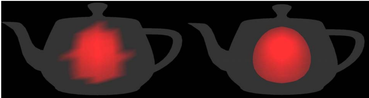
Teapot with per-vertex and per-pixel lighting using a spot-light
