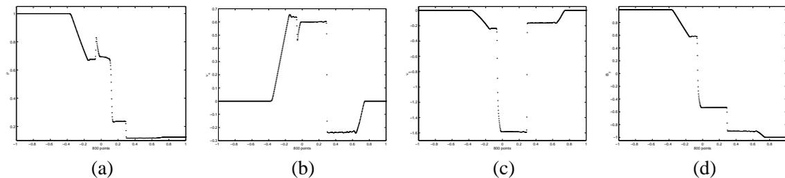
FIGURE 1. Results of Brio-Wu one-dimensional MHD shock tub computed with Jacobian free form of 3rd order Liu-Tadmor fully-discrete scheme. (a) density, (b)  $x$ -velocity, (c)  $y$ -velocity, (d)  $y$ -magnetic field
