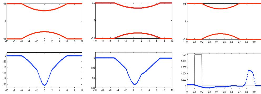
FIGURE 4. Steady-state solutions of shallow water flows. Top figures channel width, bottom figures total water height. Left: smooth flow through a channel with a centered contraction and bottom topography. Center: smooth flow through a channel with same contraction shifted to the right. Right: flow of a perturbation from steady-state of rest through a contraction shifted to the left – black line represents initial perturbation.
