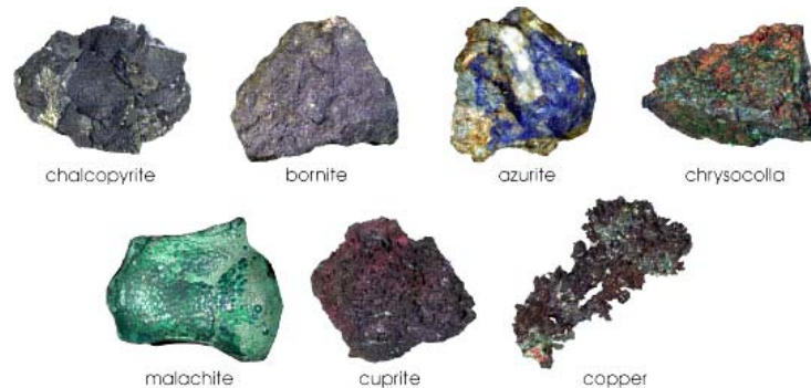
Figure 22: Example of copper ores that would have been mined by the ancient Chinese [48].
